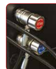
Quick couplers SAE J639 Hybrid function
